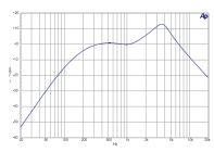
Figure 28. Digital Analyzer F-weighting curve.
