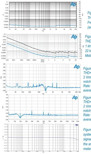
Figure 1. Typical system THD+N versus Frequency at 2 Vrms (analog sine).
