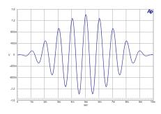
Figure 30. Shaped Sine Burst signal. (1 kHz, 10 cycles)
