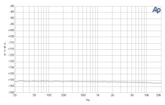
Figure 31. Typical Digital Domain system residual THD+N showing components below –140 dB.
