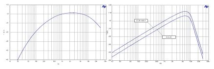
Figure 7. FIL-AWT. ANSI-IEC "A" Weighting Filter.
