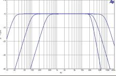
Figure 6. Typical responses of the standard bandlimiting filters.
