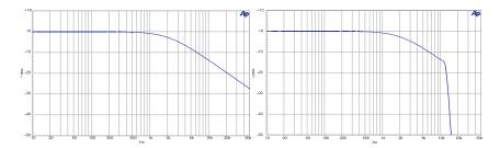
Figure 14. FIL-D75. 75  $\mu$ s De-emphasis Filter.
