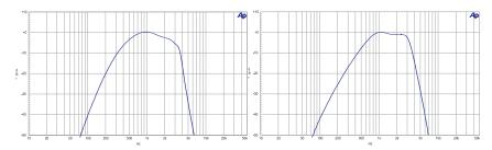
Figure 9. FIL-CIT. CCITT P53 Noise Weighting Filter.
